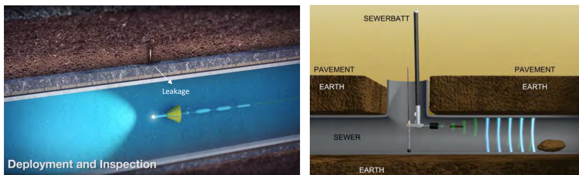
Figure 3: A typical inspection system: (left) in clean water pipe using hydrophone and CCTV (provided by Pure Technologies Ltd (2019)); (right) in sewer pipe using a speaker and microphone array (Bin Ali et al., 2011).
