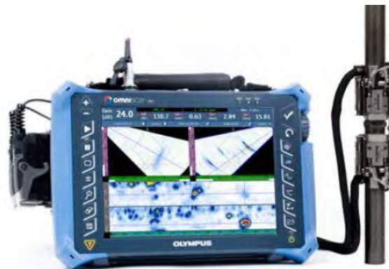
Figure 6: Commercial array imaging system in which an externally mounted 1D array is swept through a range of angles to inspect a weld (Olympus Industrial Resources, 2019).
