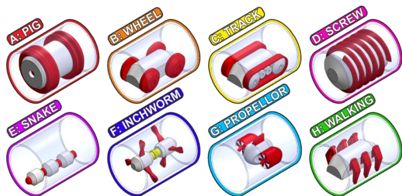
Figure 2: Locomotion techniques within pipes
