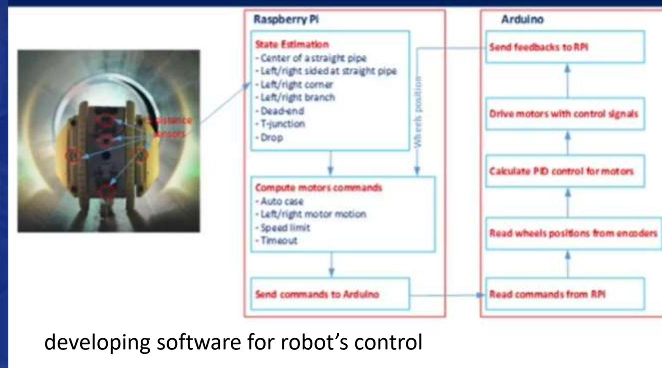
Developed low-level robot control to cope with noise and sensor inaccuracies.
