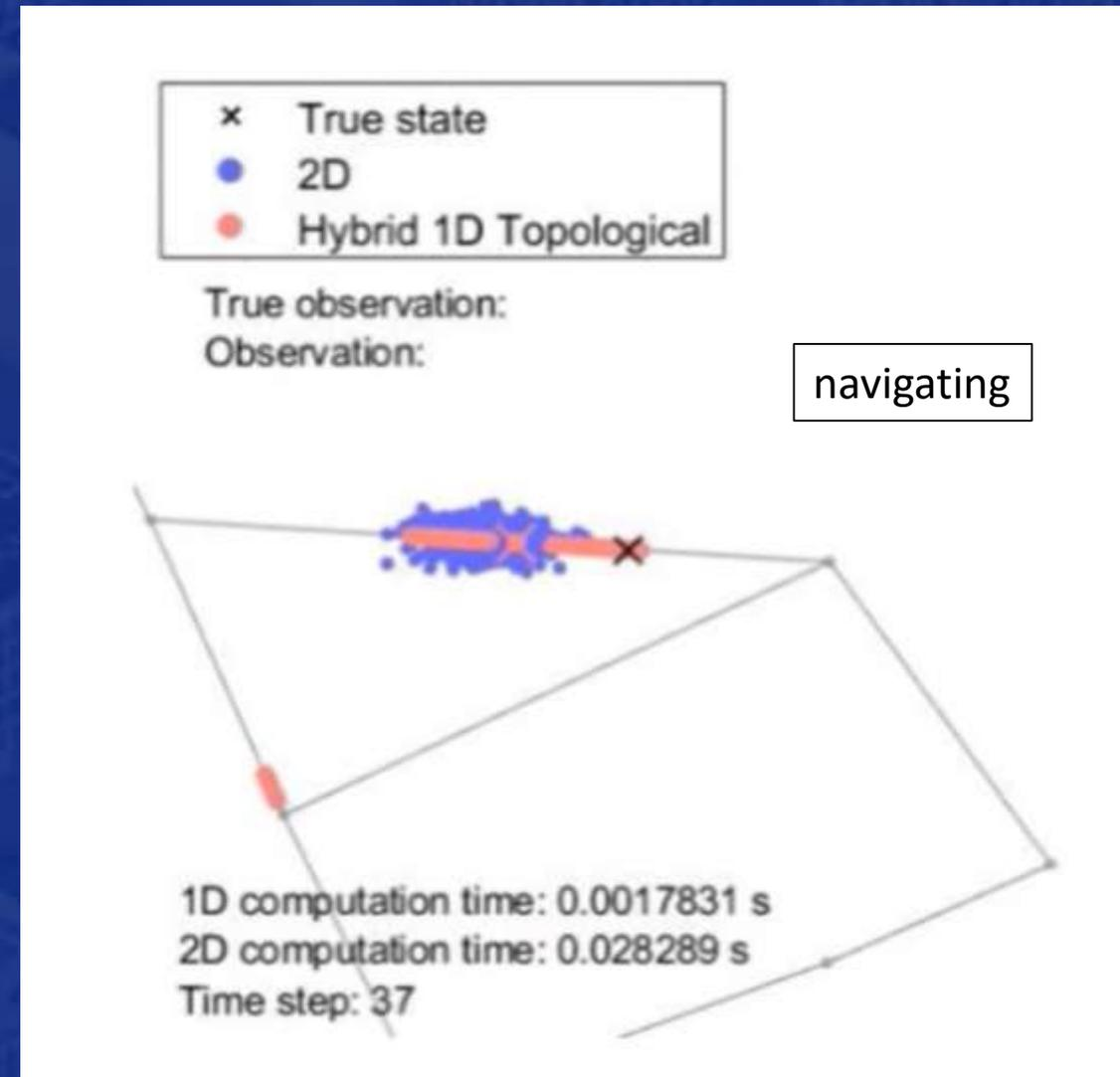
Developed algorithms for mapping & robot localisation in pipes using visual & acoustical data. Tested these algorithms through simulation and in the iCAIR laboratory.
